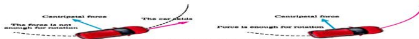
Fig. (183) : If the centripetal force is not sufficient, the car will skid out of the curved path.
